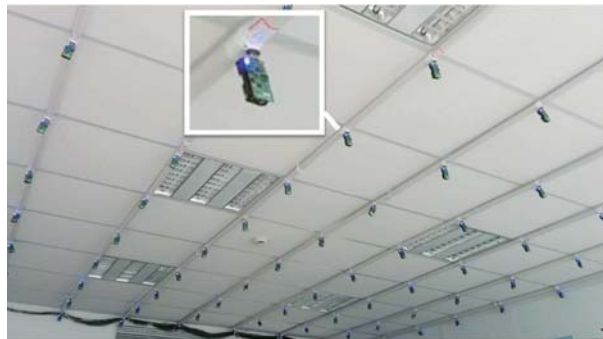
Fig. 7: The 8 \times 10 testbed with TelosB/TinyOS nodes.
